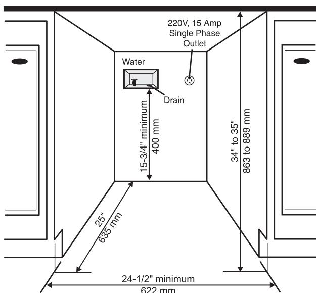
If the drain outlet is higher than 24" (610 mm), the connections will need to be recessed.
