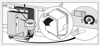
4 Adjust the front feet by turning them clockwise to raise and counterclockwise to lower the dishwasher.
