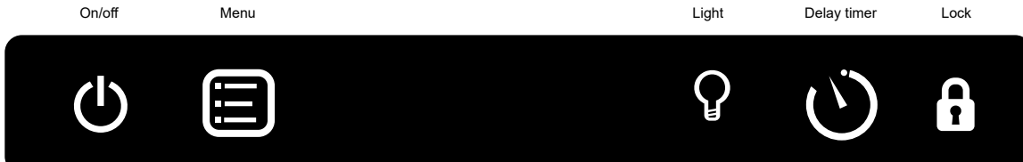
Figure 12: User interface display during power interruption.
